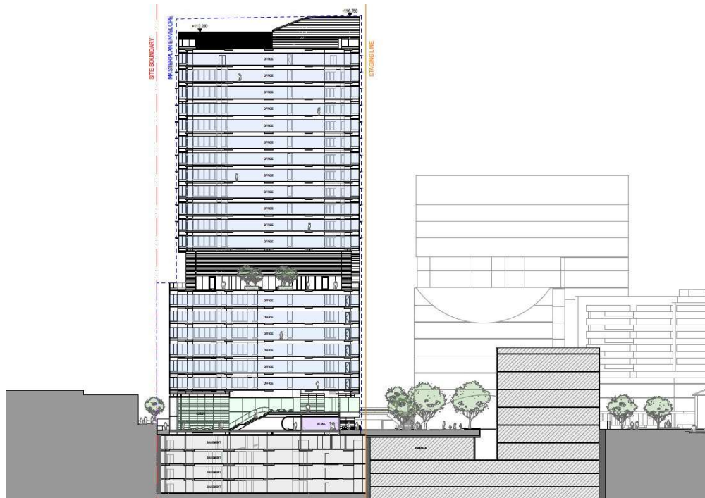
Figure 36 - East West Section through the commercial building, again showing the level 6 and 7 terrace, the setback at ground level to the podium and the basement garages below. (Source: FJMT Architects)
