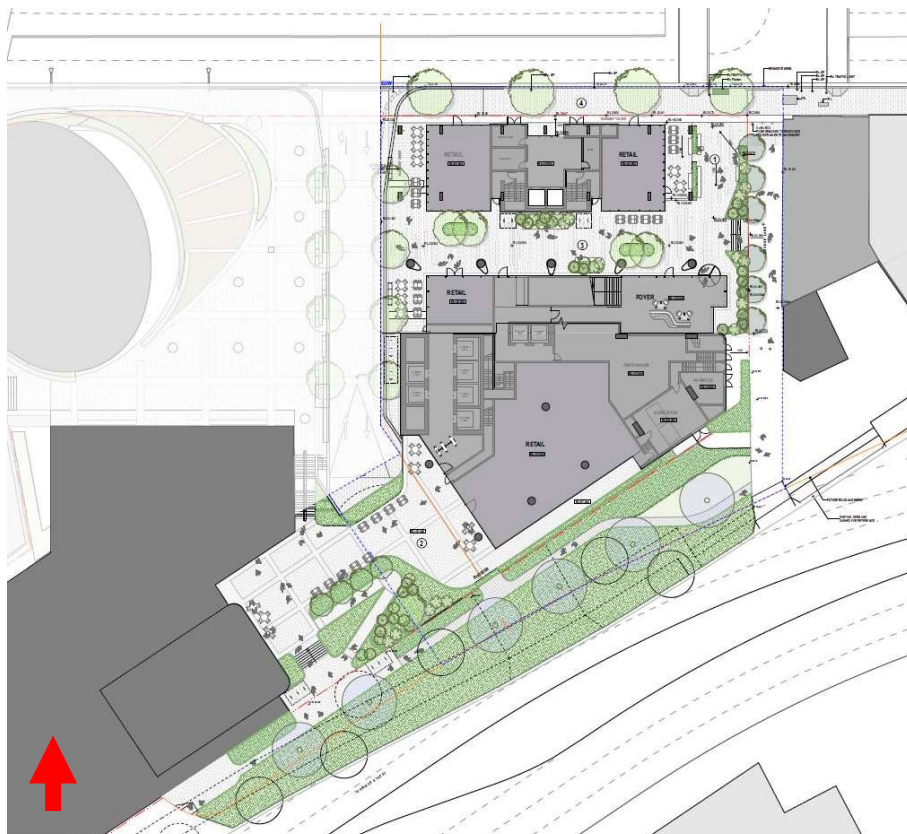
Figure 33 - Ground level plan showing the layout of the pedestrian level retail tenancies and landscaping proposed for the through site link areas and along the Terminus Street frontage associated with Phases Band C. (Source: FJMT Architects)
